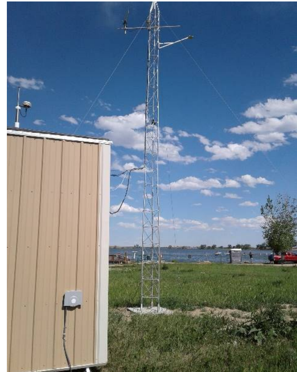
LUR instrument shelter with adjacent meteorological tower
